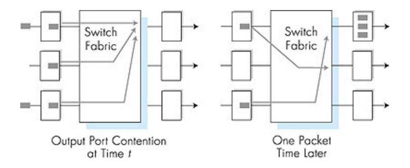
buffering when arrival rate via switch exceeds output line speed
