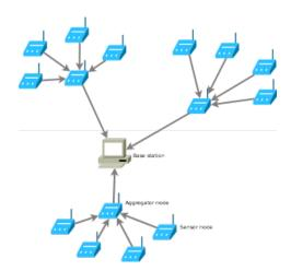
Figure 1: Structure of a wireless sensor network
