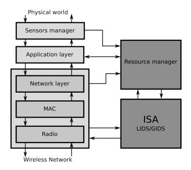
Figure 3: The node component graph with ISA added
